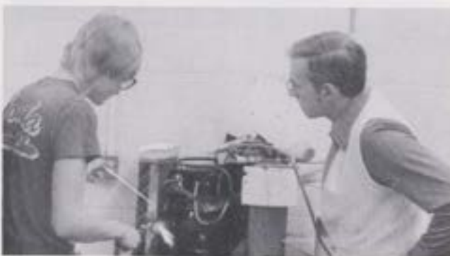
Mr. Jerry Killinger, Instructor, watching Keith Rodgers solder tubing on window air conditioner.
